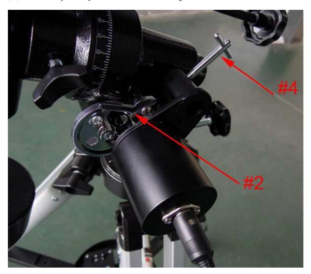
6. As soon as you have connected the motor drive to the battery box and the hand controller it is ready to use. If you want to drive your telescope by hand, please turn the clutch (#2) into opening position and use the flexible cable control.
