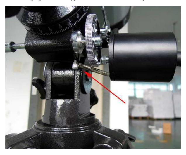
4. Then install the motor drive to the support (#3) as the following picture shows. You might need to pull back the motor drive a little bit harder due to the spring that holds the gears in position.
