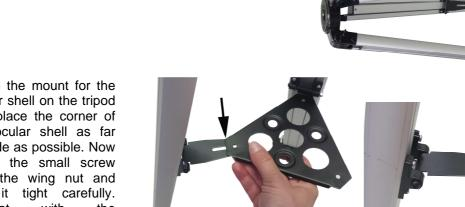
Raise the mount for the ocular shell on the tripod and place the corner of the ocular shell as far outside as possible. Now insert the small screw with the wing nut and pull it tight carefully. Repeat with the remaining two brackets.
