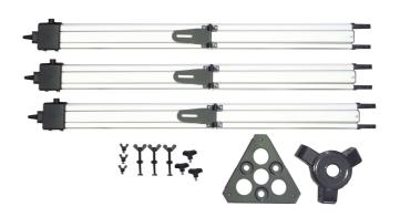
At the tripod mount there are three mountings. Take one tripod leg and slide the upper connecting piece carefully to the mounting of the tripod mount. Ensure that the holes for the screws are at the same spot. You can simply take a look from the side to see if the holes are aligned fittingly.
