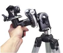
Rotate the declination axis of the mounting upwards, if needed, and attach the telescope tube ring. To do that, unscrew both screws from the mounting socket for the telescope tube ring.
