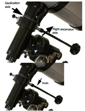
If you've adjusted and aligned the telescope correctly, then the advantage of this paralactic mounting is that you now can only track the celestial objects through the fine movement with the shafts.
