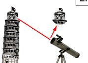
Look through the viewfinder tube. If you do not see exactly the same image, adjust the viewfinder tube. On the search tube you will find small screws, which can be used to adjust the viewfinder tube until the object can be seen exactly in the viewfinder tube. Then you have aligned telescope and finder telescope parallel to each other. If you encounter the viewfinder, repeat the procedure.
