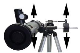
Depending on if the tube or the counterweight sinks down, move the counterweight on the rod to achieve a balance.
