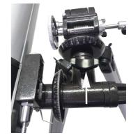
The side of the telescope tube or the side of the counterweight will now probably sink downwards. It depends on which side is heavier.
